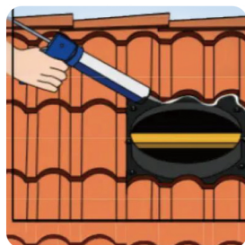
③ Secure and seal the flashing
