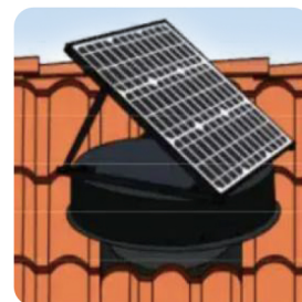
⑤ Connect cables & adjust the solar panel angle
